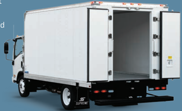
(Shown with optional insulated double-narrow swing rear doors and reefer access steps)
