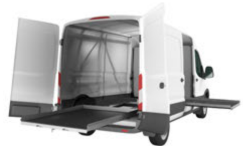
WALLSLIDE Systems are compatible with CARGOGLIDE units that pull out the rear and side of your van.
