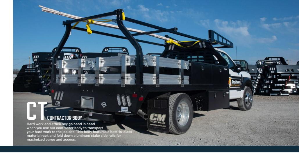
FEATURES AND OPTIONS LENGTHS 9'4", 11'4" HEADACHE RACK Steel Tube Clear LED Oval HEADACHE RACK LIGHTING DECK 1/8" Treadplate FRAME RAILS 4" Structural Channel Steel CROSSMEMBERS 3" Roll-Formed 3/16" Channel Crossmembers REAR SKIRT Solid One Piece with Rear Step GN HITCH BP HITCH 24K lb. 2 1/2" B&W Hitch with Receiver Tube SIDE RAILS 3/8" x 2" Side Rails with Stake Pockets
