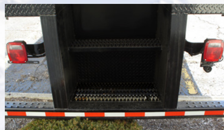
Dock Extension with Two-Step Center Stairway
