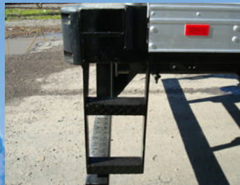
Steel Stirrup Step on Dock Extension
