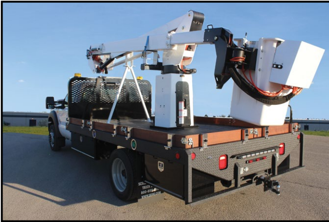
Pictured above is ATA Device on Scelzi 8 x 14 flatbed, WO #108160. Body has PTO and pump for boom lift, back up alarm, basket capacity of 400 lbs, and 540 degree boom rotation with mechanical stop. Meets or exceeds ANSI A92.2-2001 and OSHA requirements
