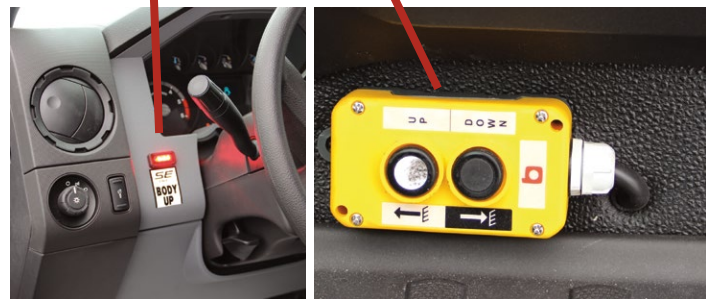
Dash-mounted LED "Hoist Up" Safety Light and Push Button Hoist Up-Down Controller
