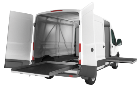
WALLSLIDE Systems are compatible with CARGOGLIDE floor units that pull out of the rear and side of your van.
