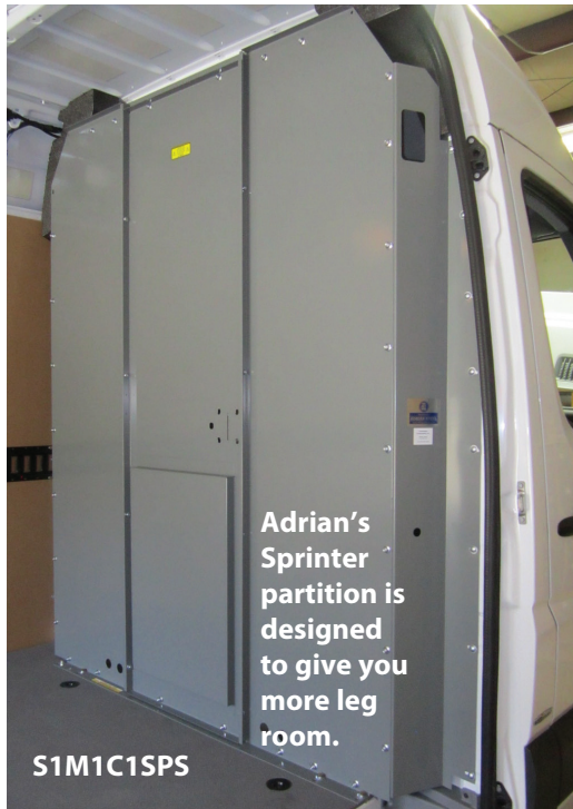
PDK2 Steel Partition Door Kit converts fixed center panel partition into a hinged door with keyed handle.
