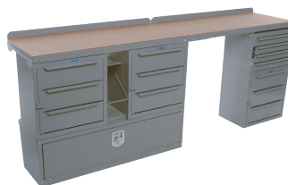
MD610 Workbench Module includes a heavy-duty steel workbench with a Masonite covered worktop, stool, nine lockable medium drawers, four locking shallow drawers, a catalog file and a lockable wheel-house cover. Measures 84" W, 32" H, 12"/18" D.
